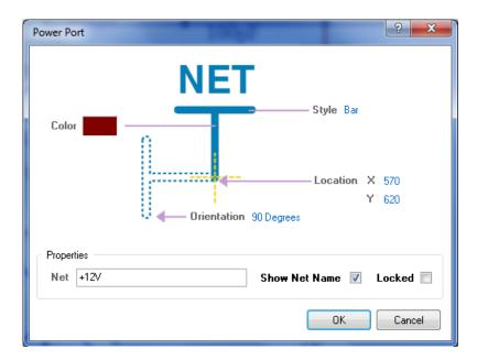
b. Click the 'GND Power Port' button next to the 'Place Wire' button and place (6) of them in the schematic in the places shown in the image on the next page
