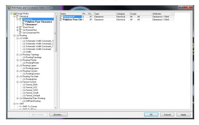
Click on the new rule on the left column. This will display the properties on the PolyGon Pour Clearance rule.
