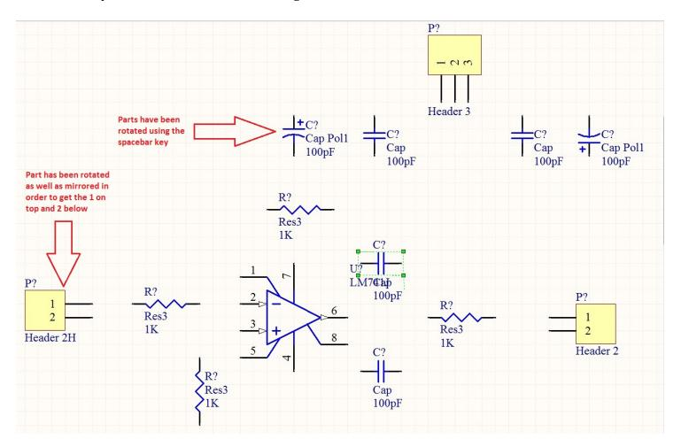
**Notice:** The 'Header 2H' part has been rotated as well as mirrored in order to get the 1 pin on top when the part is in this orientation. Rotation is accomplished with the **spacebar** key while the mirror is added by right-clicking the part and checking the 'mirrored' checkbox. This does not make any difference on the PCB file it just makes your schematic easier to view and understand.
