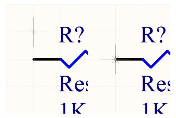
The image to the right is connected properly. The X in the crosshair has turned red showing that a connection is being made.
