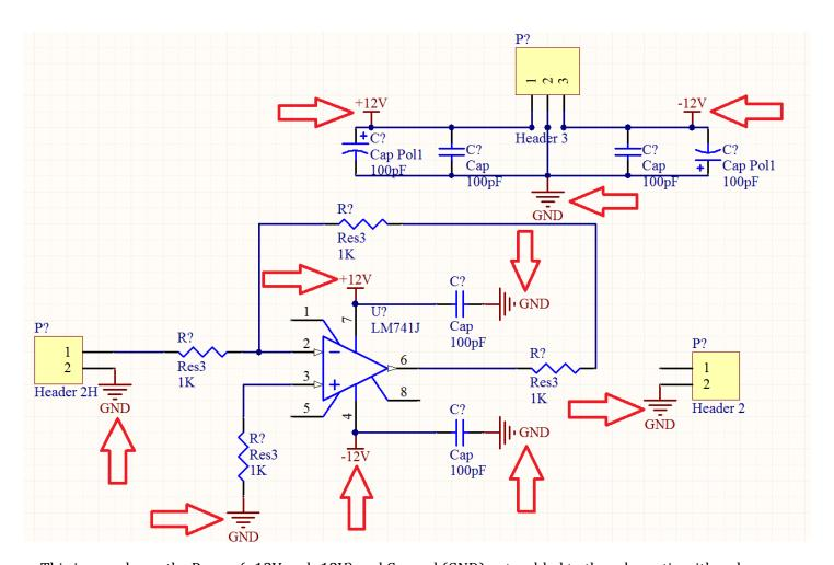
This image shows the Power (+12V and -12V) and Ground (GND) nets added to the schematic with red arrows
