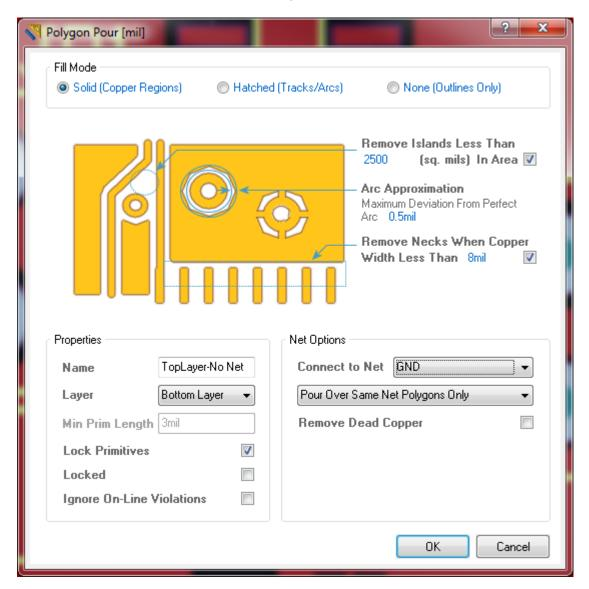
The bottom layer should be selecter as well as the connection to the ground net.
