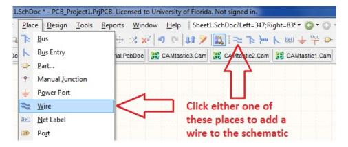
b. Once you click this icon your cursor will turn into a crosshair with a black X on it. Once you hover over a valid place to connect a wire the X will turn red. If the X does not turn red when you place the wire a proper connection was not made and this will lead to errors later in the process. The red X is illustrated close up below.
